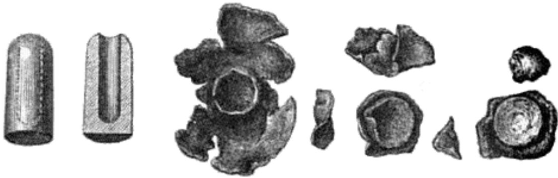
Cross sectional views of the Dum-Dum Bullet
